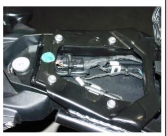
Reusing the original bolts, fit the L-Brackets to these points as shown in Diagram #2, leave slightly loose.
